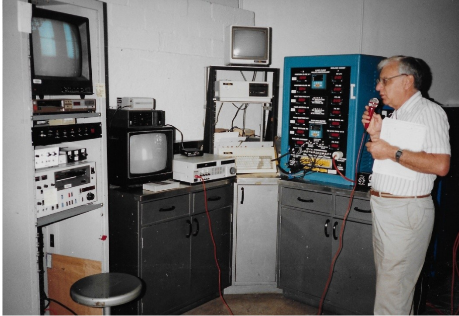
Stan Glickstein operating his neutron radiography data acquisition apparatus at the Penn State University nuclear reactor.
