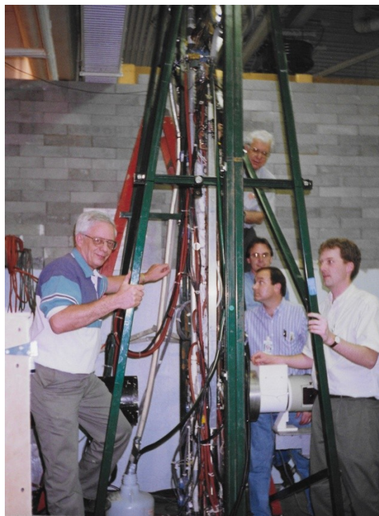
Experimental loop for studying vapor flow in boiling water using neutron radiography
