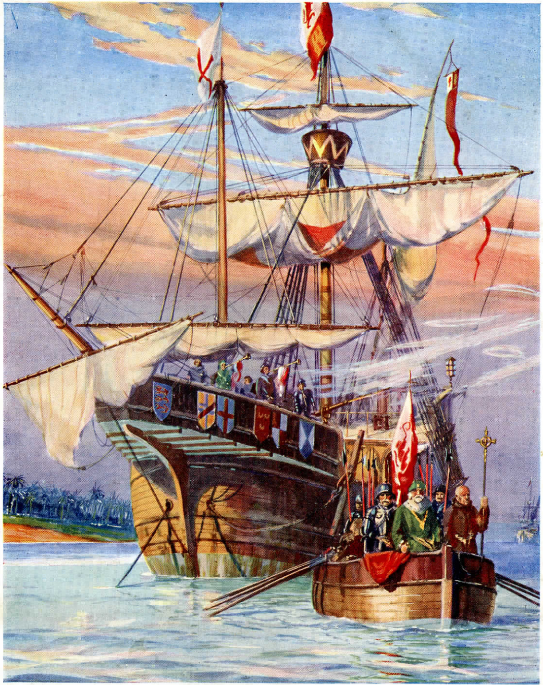
"Santa Maria," The Flagship of Christopher Columbus, 1492. Length of ship, proper, 93 feet. Beam 25-71 feet. Displacement 233 tons.
